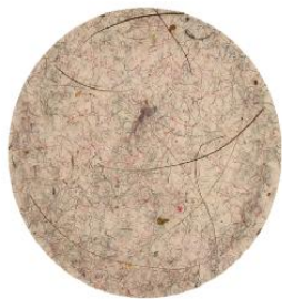
Fig.1. Condensed water from a tumble dryer from one washing (47 mm diameter filter of 1 µm).
