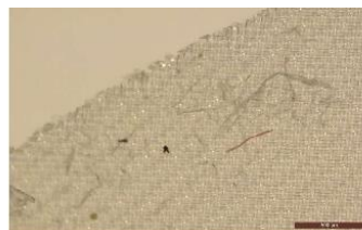
Fig.6. Surgical mask migration experiment, where MP released from the mask are preconcentrated on 25 mm filter of 25 µm.
