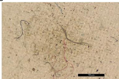
Fig.5. Bus indoor air, 180 m 3 preconcentrated on a 25 mm filter of 25 µm.
