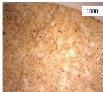
Fig.2. Two and a half L river water filtered on a 47 mm filter of 1 µm.
