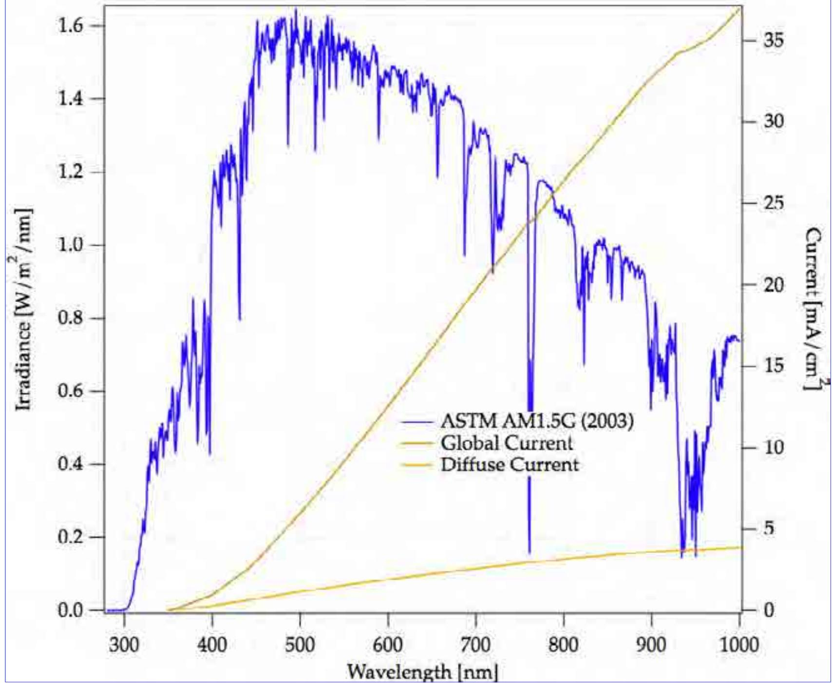
The DX1 dye harvests more near IR light in the 750 -900 nm region than the black dye
