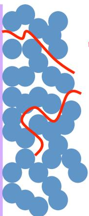
Transparent layer: 5 $\mu\text{m}$  of 20nm particle, 32nm pore size
