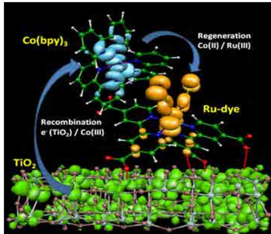
Schematic representation of the higher recombination probability of N719 with respect to the Z907 dye with cobalt electrolyte.
