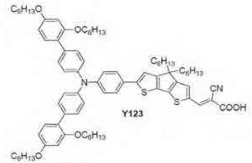
DSCs consisting of a 5.6  $\mu\text{m}$  thin transparent nanoporous  $\text{TiO}_2$  (anatase) film, the Y123 sensitizer.
