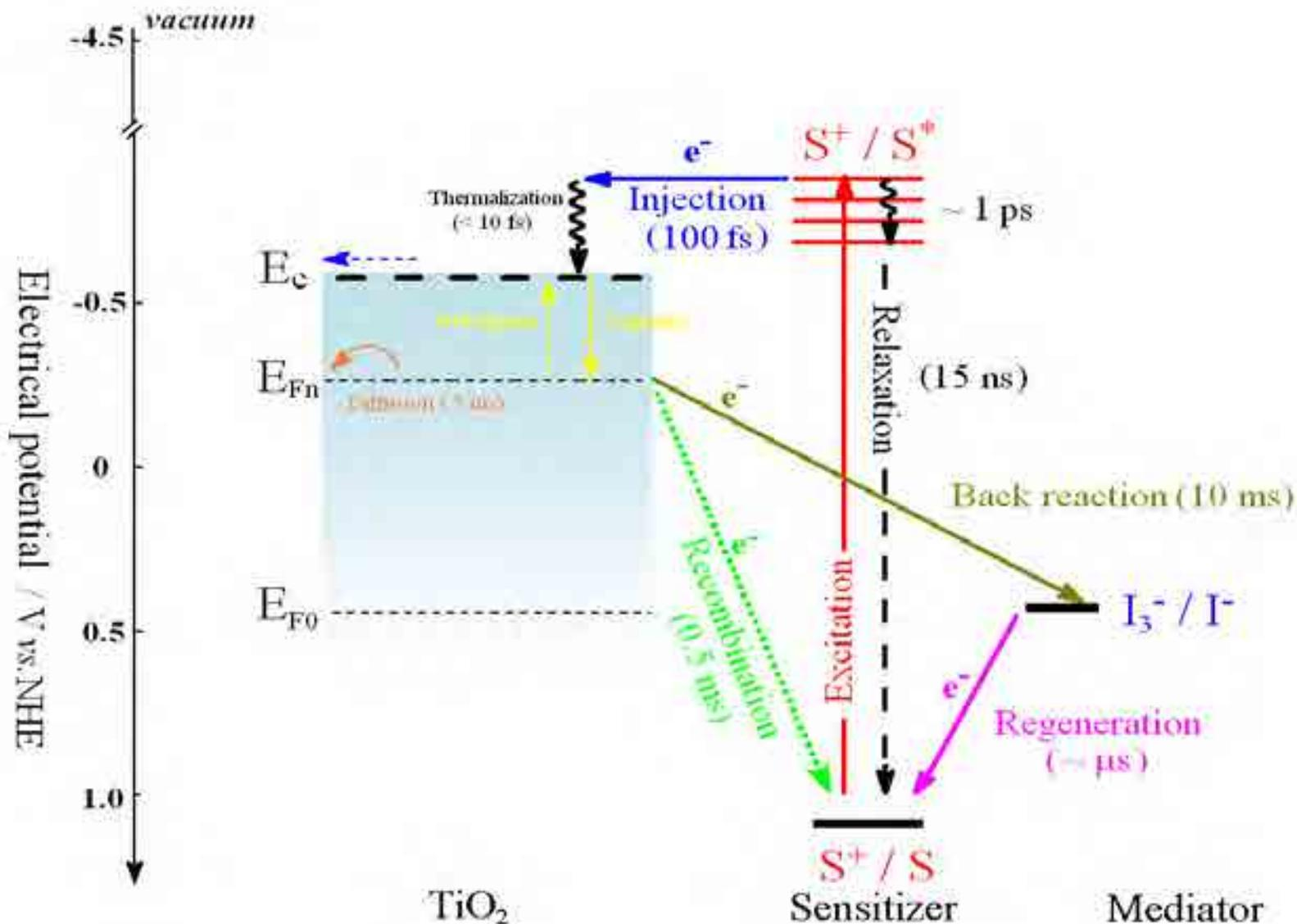
Photo-induced interfacial charge separation occurs within femtoseconds
