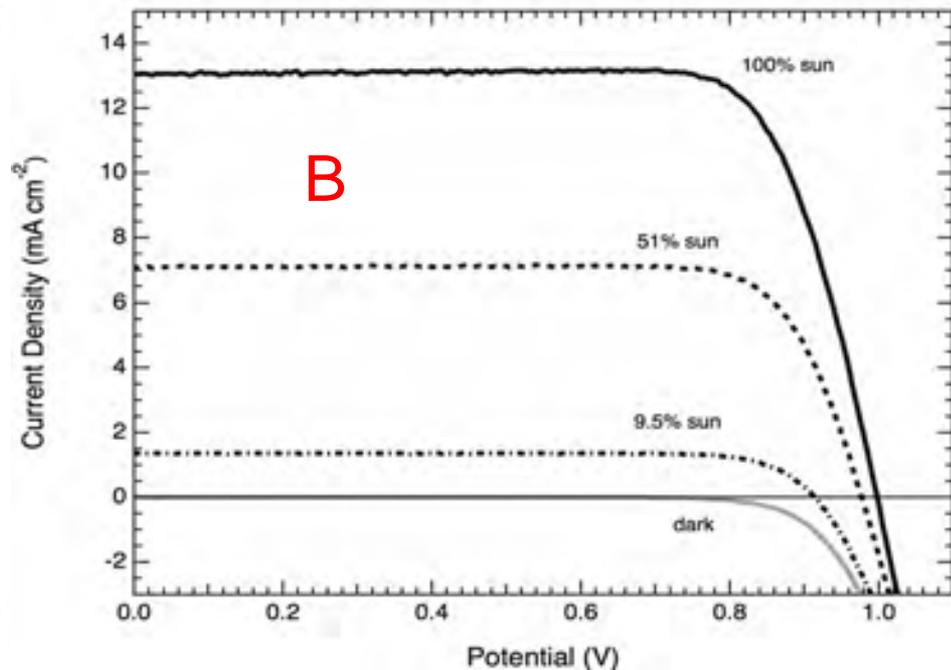
**Photovoltaic characteristics of DSC based on  $[\text{Co}(\text{bpy-pz})_2]^{2+/3+}$  system**
